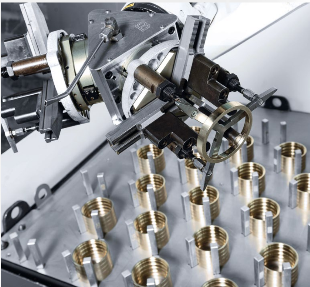
The Robo2Go stacking magazine offers sufficient capacity to enable around-the-clock production with the CTX beta 800 TC.
