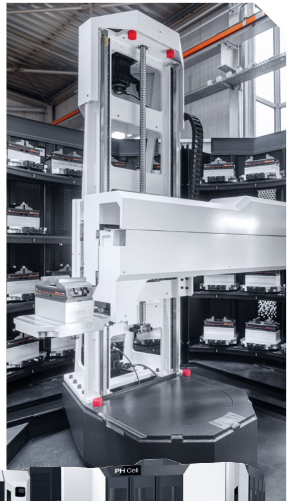
The DMU 50 3 rd Generation is loaded from the side, which offers optimal accessibility to the machine and automation. The PH Cell is equipped with a total of 40 pallet storage positions.
