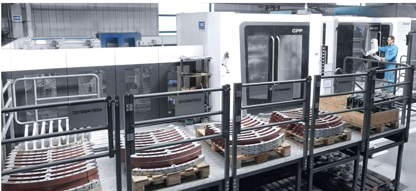
Trützschler uses an NHX with a 7-station carrier pallet pool (CPP) for automated manufacturing of large components.
